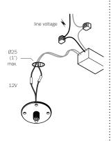
Connect power supply to line voltage.
