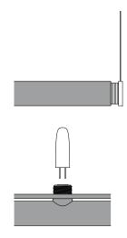
Thread the stem onto the connector that is located at the end of the coax cable.
